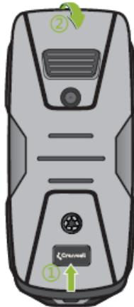
**Note:** If the battery is inserted, remove the battery by lifting it using the finger grip.
